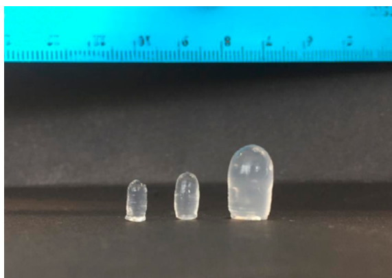
Fig. 2 illustrates the appearance of the solid rectal formulations printed using the hydrogel compound of a 6 % of Laponite XLG. The high resolution in the printing process allowed printing designs of different sizes.
